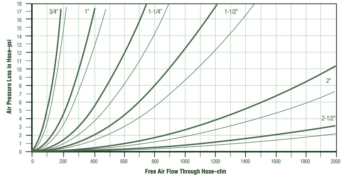
**Example #1:** A customer has a 185 cfm air compressor equipped with 100' of 3/4" hose to operate a Sullair 90 pound paving breaker. The 90 pound paving breaker requires 62 cfm to operate. How much pressure loss can the customer expect at the tool if the compressor is providing 100 psig inlet pressure?
